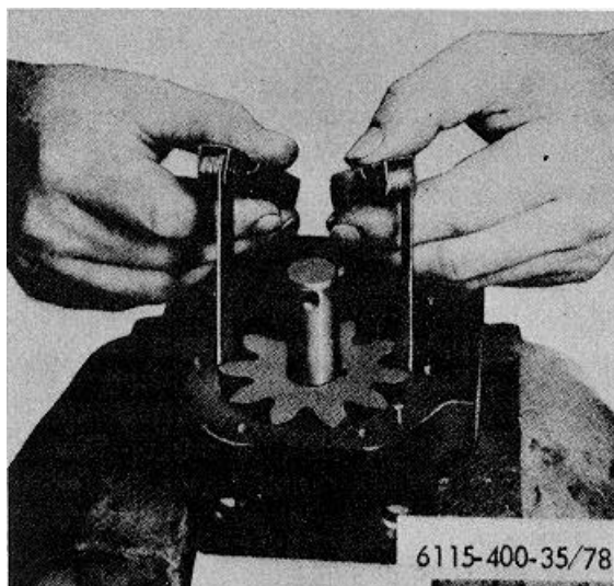
Figure 78. Checking radial clearance between gear teeth and pump body.
